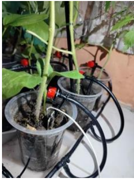
Gambar 9 Sensor Sensor Soil Moisture Mendeteksi Kelembaban Tanah
